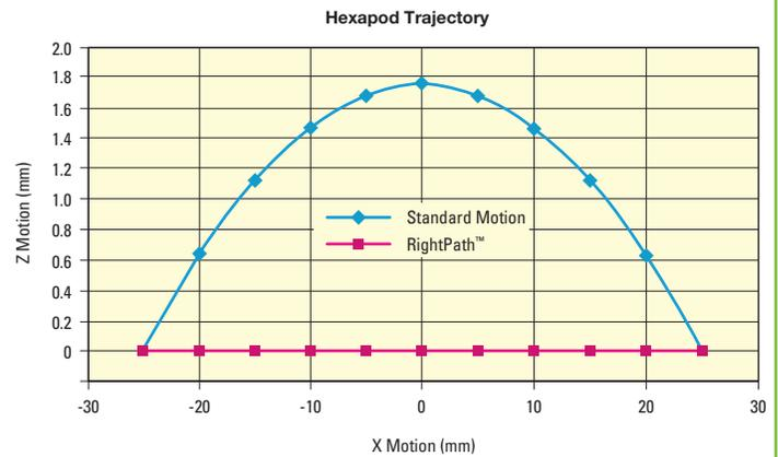
RightPath™ Trajectory Control enables minimal runout in linear and arc trajectories.
